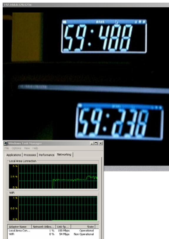
Figure 12. Streaming using the Java media framework, 320x240 30fps, MJPEG coding, delay 150ms, bandwidth use: 2.5 Mb/s
